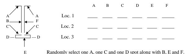
**B.** Two random adhesion tests per span are conducted on interior surfaces after the paint has been properly cured, and will be touched up by the Contractor. One random Cut Tape adhesion test per span is conducted on interior surface after the finish coat is cured, and will be touched up by the
